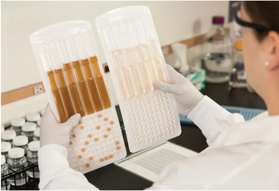
The IDEXX Legiolert test indicates samples contaminated with Legionella pneumophila by turning a caramel brown colour after seven days' incubation.
