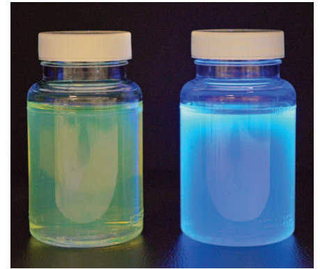
The IDEXX Pseudalert test shows a positive indication for Pseudomonas aeruginosa (fluorescence under UV light on right) after 24-hour incubation in a presence/absence test.
