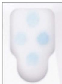
Because protein-conjugate binds to the sample spot only if there is little or no residue, a strong blue color (darker than the control) means a negative test result. **Note:** Number of spots may vary.
