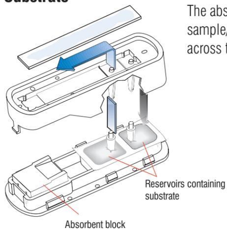
The absorbent block draws the sample/substrate mixture back across the sample spots.
