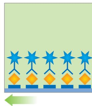
If the protein-conjugate is bound to residue in the milk, there is little or no color development in the sample spot. If the protein conjugate is bound to the sample spot, the substrate reacts with the sample spot, turning it a strong blue.
