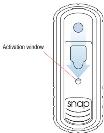
Sample flows across the test spots and activation window. When the sample passes through the activation window, the device is activated ("snapped").
