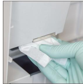
2. Open the analyzer door and clean the top and bottom of the pipetting window with a damp optical tissue. Then dry with a new dry optical tissue.
