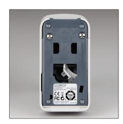
Ensure the base and silver fasteners are flush with the analyzer and locked into place. Not locking the base and fasteners properly can impact analyzer performance.
