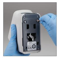
7. Turn the silver fasteners clockwise a quarter turn to lock the base into place.
