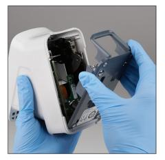
3. Remove the base from the analyzer. 4.
