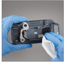
Clean the **entire** base using a lintfree wipe or cotton swab dampened with 70% isopropyl alcohol, mild liquid soap and water, or a 10% bleach solution.
