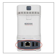
Power off the analyzer and disconnect the power and/or Ethernet cord.
