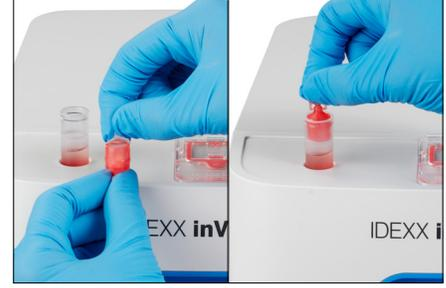
a. Pull to remove the foil seal from the sample tube.
