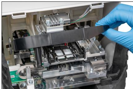
b. Lift the shutter until it locks into the raised position.
