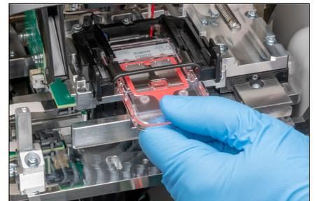
c. Carefully remove the jammed cartridge from the cartridge holder and discard. Do not reuse the cartridge.
