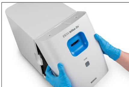
e. Replace the front cover by inserting the top tabs into the corresponding slots at the top of the analyzer until the cover and analyzer edges are touching. Then, press the bottom of the cover down until it snaps into place.
