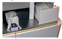
Load slide here Load tips here
