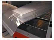
10b. Alternatively, insert tray(s) paper side down into an appropriately sized resealable plastic bag or box. Then incubate container at 37°C (±0.5°C) for 7 days. Do not remove trays from the incubator prior to the final read.
