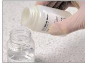
Add 100 mL of sterile diluent (e.g., deionized water, phosphate/ Butterfield's buffer, or 0.1% peptone) to a sterile vessel with no additives.
