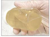
Cap the vessel and shake to dissolve. Sample may remain cloudy but can be added to the Quanti-Tray\* when no large particles are visible.
