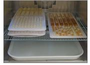
10a. Place trays paper side down into humidified incubator at 37°C (±0.5°C) for 7 days. Provide adequate humidity to minimize Quanti-Tray water loss during 7 days. Do not remove trays from the incubator prior to the final read.
