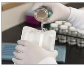
Agitate and then pour sample into a Quanti-Tray\*/Legiolert\* tray. Tap tray to remove any air bubbles from small wells.
