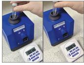
Start a 1 minute timer; then mix the contents. Keep the tube at room temperature for 60 seconds (±5 seconds). Mix the tube again before 60 seconds has elapsed.
