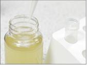
6. At 1 minute, immediately transfer only 2.0 mL of the treated sample to the vessel containing the dissolved Legiolert reagent as prepared in steps 1 and 2.
