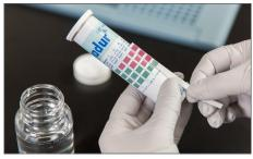
1. Bring sample to room temperature and measure hardness.
