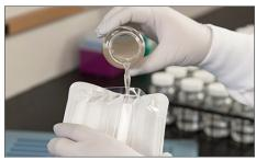
Agitate and then pour sample into a Quanti-Tray\*/Legiolert\* tray.<sup>†</sup> Tap tray to remove any air bubbles from small wells.
