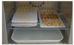
7a. Place trays paper side down into humidified incubator at 39°C ( $\pm 0.5$ °C) for 7 days. Provide adequate humidity to minimize Quanti-Tray water loss during 7 days. Do not remove trays from the incubator prior to the final read.
