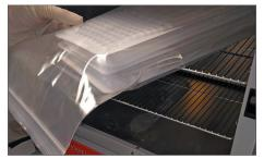
7b. Alternatively, insert tray(s) paper side down into an appropriately sized resealable plastic bag or box. Then incubate container at 39°C (±0.5°C) for 7 days. Do not remove trays from the incubator prior to the final read.
