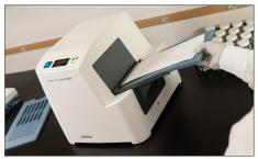
6. Immediately seal the tray using the Quanti-Tray\* Sealer PLUS.
