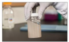
4. Cap the vessel and shake to dissolve. Sample may remain cloudy but can be added to the Quanti-Tray\* when no large particles are visible.
