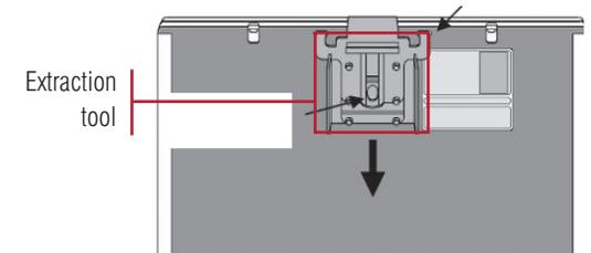
Removing the extraction tool
