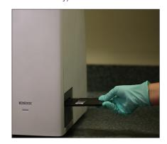
Gently insert the slide tray into the instrument until it stops (do not force it in as scan errors may result). The instrument will automatically pull in the slide tray.
