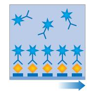
If residue is present in the milk, the protein-conjugate is not available to bind with the sample spot.
