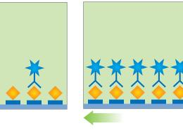
If the protein-conjugate is bound to residue in the milk, there is little or no color development in the sample spot. If the protein conjugate is bound to the sample spot, the substrate reacts with the sample spot, turning it a strong blue.
