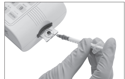
Figure 4-2: Add sample to center of well
