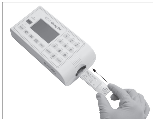
Figure 3-1: Insert cartridge, label facing up
