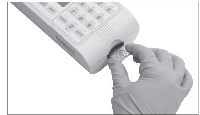
Figure 4-8: Insert Coag Dx Citrate PT or Citrate aPTT cartridge
