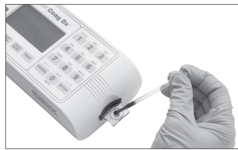
Figure 4-10: Add sample to center of well
