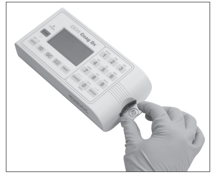
Figure 4-1: Insert Coag Dx PT or aPTT cartridge
