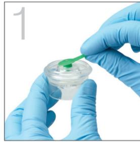
1. Remove the green cap from the lithium heparin whole blood separator to prepare it for sample collection.
