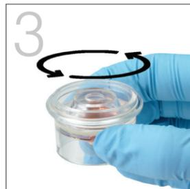
3. Gently swirl (**do not invert or shake**) the whole blood separator at least 5 times to mix the sample with the anticoagulant.
