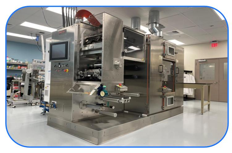
R&D Catalyst Slide "Coater": Direct simulants of manufacturing lines
