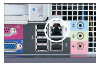
Ethernet port on the back panel of the IDEXX VetLab Station computer's CPU
